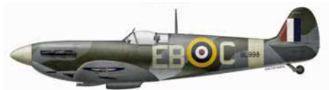
Supermarine Spitfire EB-C as flown by Sgt Goodall. Armed with two Hispano 20 mm cannons and four Browning.303 machine guns it could also carry two 250 lb or one 500 lb bombs. Powered by a Rolls Royce 45 series V12 engine that developed 1,440 HP
